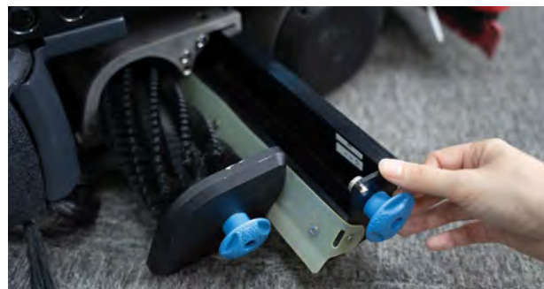
Easy Pull Out Debris Hopper & Brushes
